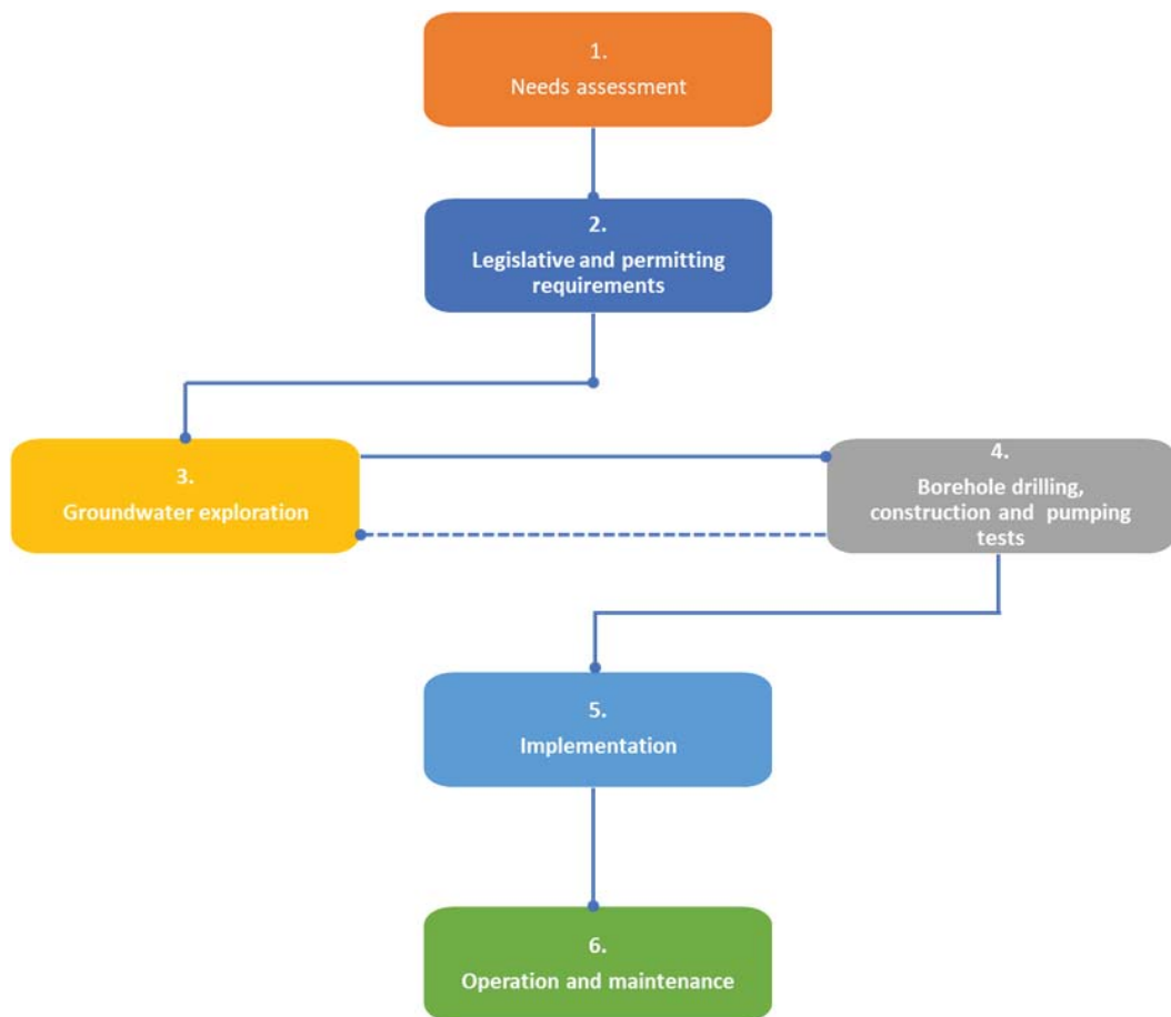
Figure 2: The five life cycle stages of a water and sanitation development project. Solid arrows indicate the flow of the life cycle process. The dotted arrow indicates the potential for interaction between stages 2 and 3 (after McConville and Mihelcic, 2007).
