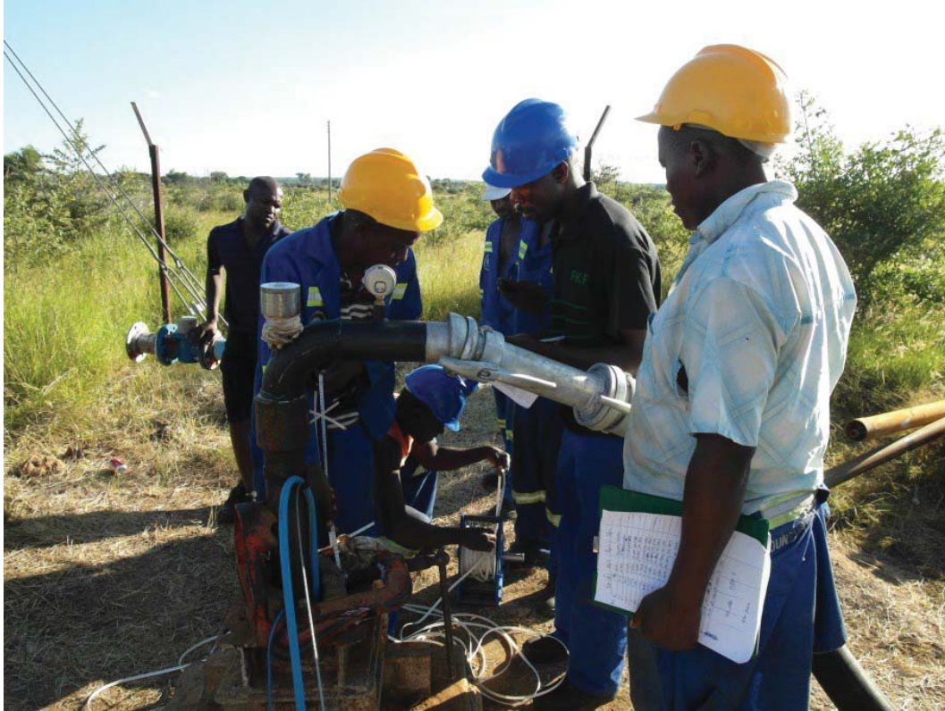
Figure 15: Taking water level readings
