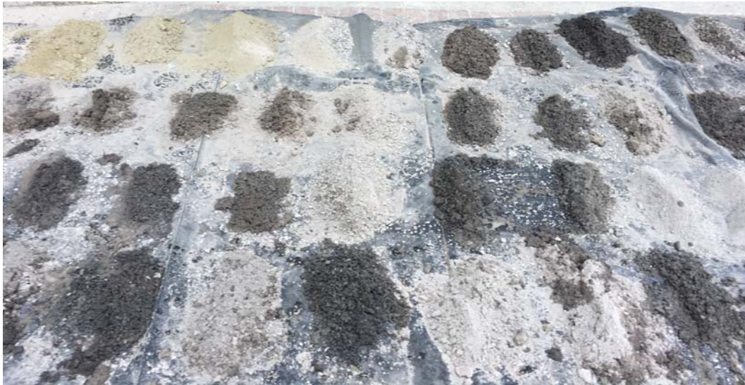
Figure 9: Drilling cuttings laid out at 1 m intervals
