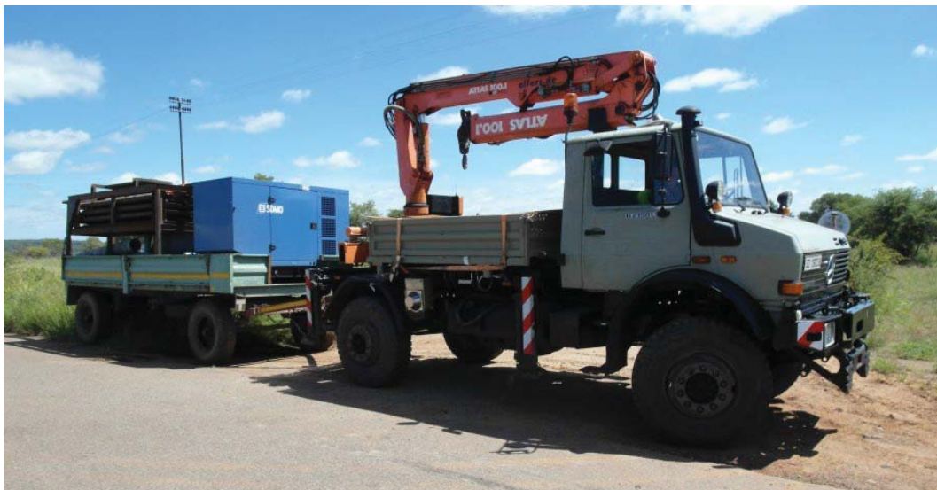
Figure 12: Unimog with crane and trailer with pumping test equipment for Nyamandhlovu pumping tests (photo credit: Hans Beekman)
